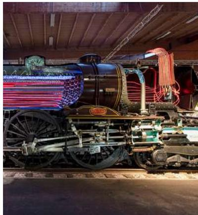
At the Cité du Train, we explain to you how such a heavy steam engine can move forward. An "open" locomotive presents its main organs. Another one sets into motion every 30 minutes to show how connecting rods work. You can look underneath it thanks to a pit.
